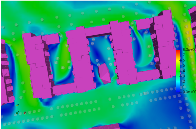
Figure 6.36: Block D/E Podium - Flow Velocity Results at Z=1.5m above the Podium - Wind Direction: 315°
