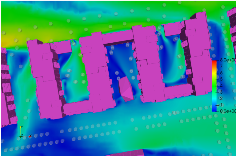
Figure 6.37: Block D/E Podium - Flow Velocity Results at Z=1.5m above the Podium - Wind Direction: 281°
