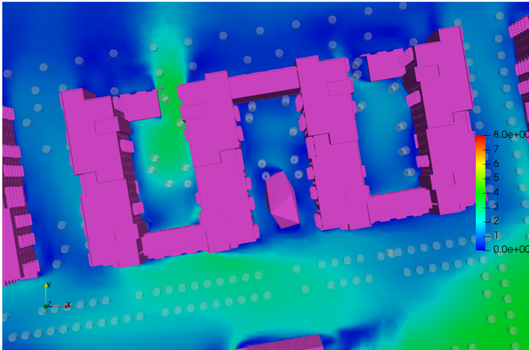
Figure 6.30: Block D/E Podium - Flow Velocity Results at Z=1.5m above the Podium - Wind Direction: 225°
